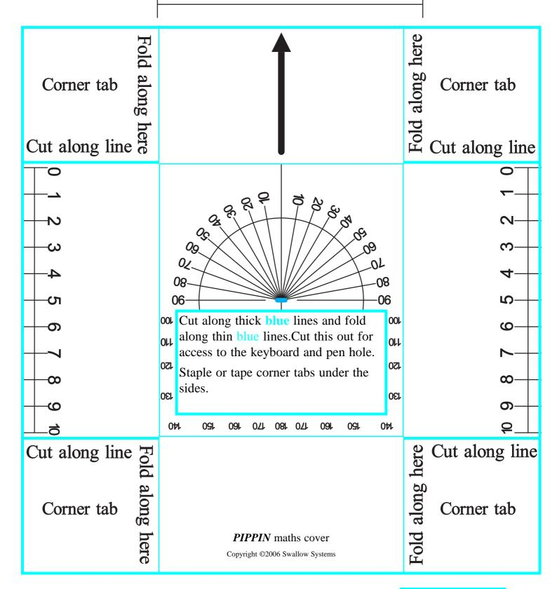
Make sure that the slot for the fastener is cut parallel to the edge of the keyboard hole. The centre of this hole must go at the centre of the protractor. The blue dot in the pointer must be round and just the right size for the fastener. The pointer
